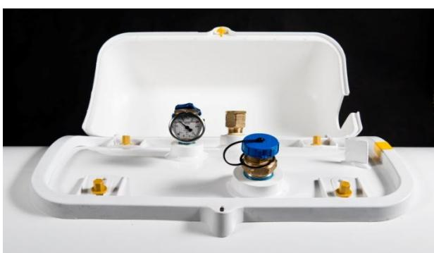
After leaving the oven is carried out the assembling of safety instruments by the reduction and pressurization kit for the next test of the sealing tools and the assembly of the cockpit instrument watertight. The pressurization of the tank is carried out at 7 bar with adequately dried air, in order to avoid that the moisture present in the air can condense on the inside of the tank. The tanks are then discharged from the chain for mounting the final accessories.
