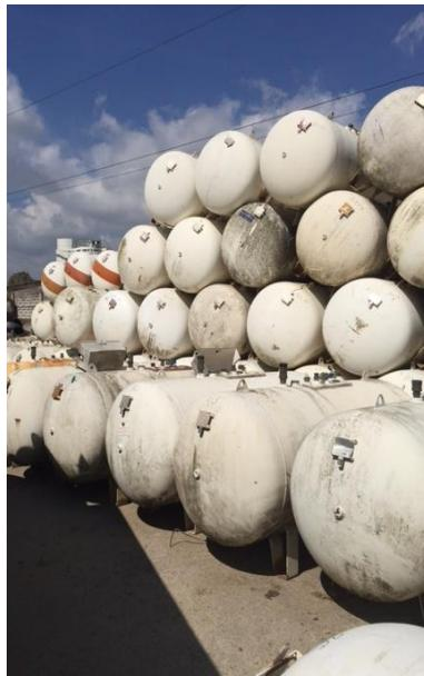
The incoming tanks for reconditioning, are deposited in a special area to proceed to depressurization and dismantling of all the accessories, and then be picked up and carried to the subsequent processing stages.
