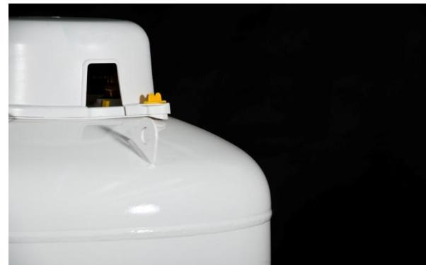
LPG AboveGround tank surface finish is made by one coat of zinc primer and one coat white polyurethane enamel paint for aboveground tanks, and epoxidic paint for the underground. The minimum thickness of the iron is 4.5 mm both on the plating and on the bottoms.
