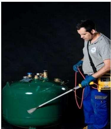
Completed assembly making the following checks, laid down in Circular P2004 Interior Ministry, by the trained and certified and calibrated instruments. For the release of the results of these verifications tanks must conform to the provisions of the circular P2004.
